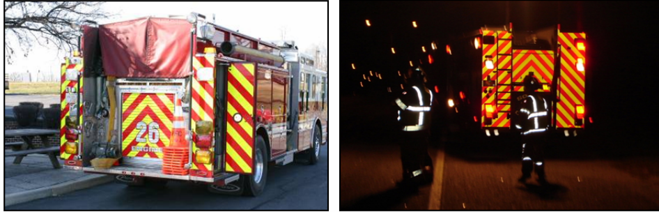
Figure 1 - Emergency Vehicles with Retroreflective Chevrons (Source: ResponderSafety.com)
